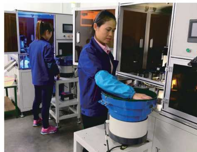
轴承内外环尺寸测量视觉检测系统/Bearing inner and outer ring dimension measurement visual inspection system
